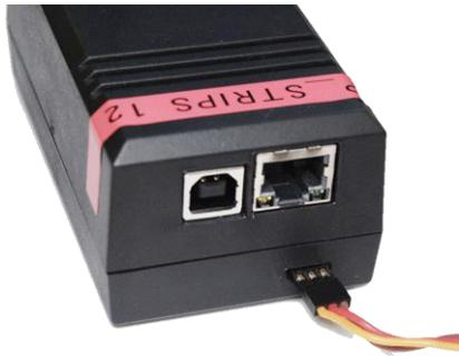
**Figure 4: Central Unit for data readout with an ETHERNET interface**
