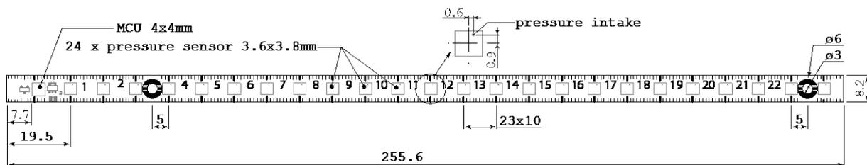
**Figure 2: Outline dimensions of the Pressure Strips**
