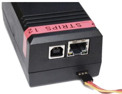
**Figure 3: Central Unit for data readout with an ETHERNET interface.**
