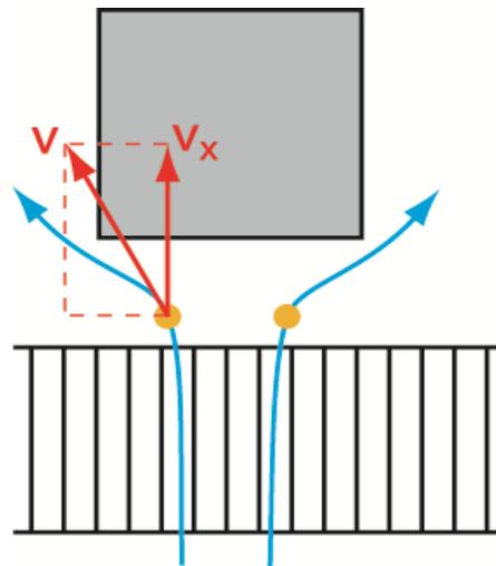
Figure 3: Flow needs to be perpendicular to the control plane
