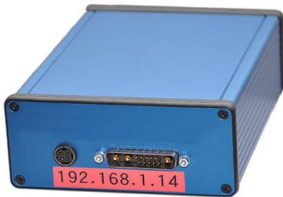
**Figure 5: Central Unit for data readout with an ETHERNET interface**
