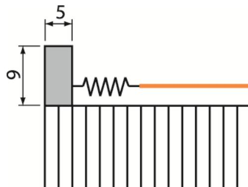
Figure 4: Rim of the sensor is only 5x9mm
